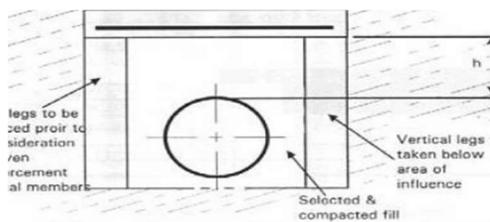
**Figure 2 (b) - Concrete Slab with supports**
